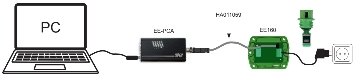
Fig. 13 EE160 configuration analogue output using EE-PCA kit
