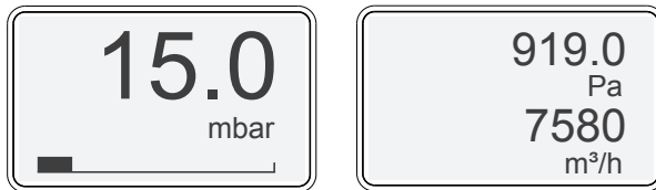
Fig. 16 Display with one line with limit bar and two lines without limit bar
